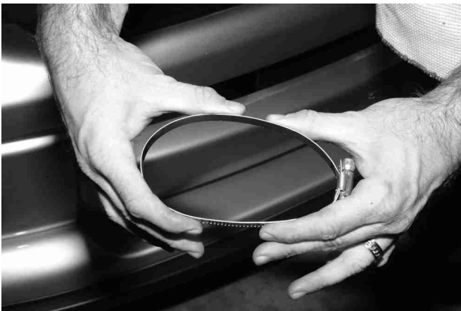
Bend hose clamps as shown to make install easier .
