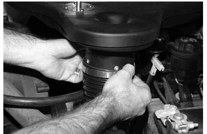
Bend hose clamps as shown to make install easier .
