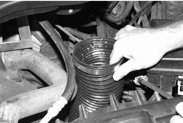
Install supplied hose and trim to reduce any unwanted slack.
