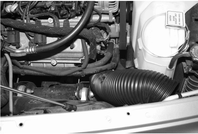
Route between frame rail and water hose just in front of control arm as shown for 1500
