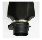
Your stock MAF will insert directly into the rear of the VR duct (years 2001-2004), If you have an early car 1997-2000 you will do the same, however, you will use duct part number VRD2. The MAF will insert firmly tighten
